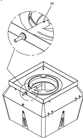
If an FRx-AFD flange is used: Remove the plug from the pipe, and insert the sensor. Tighten the screw (A).
