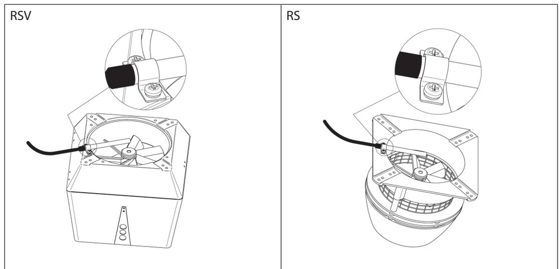
If an FRx-AFD flange is used: Remove the plug from the pipe, and insert the sensor. Tighten the screw (A).
